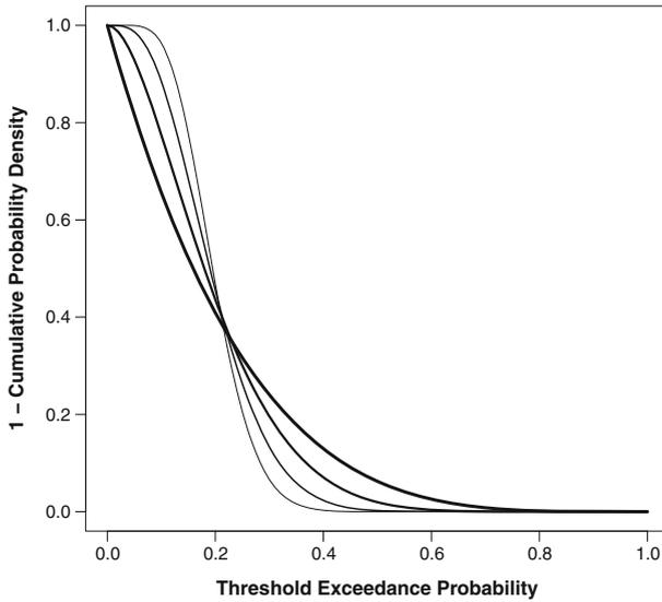
**Fig. 5** Family of complementary cumulative distribution functions for Beta distributions of constant mean ( $\mu_B = 0.2$ ) but differing variance. The standard deviations of the functions range from  $\sigma_B = 0.062$  for the lightest line, to 0.087, 0.121, and 0.163 in increasing order of line thickness
