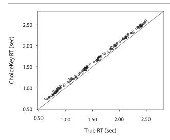
Figure 2. Response time (RT) as recorded by ChoiceKey (*y*-axis) as a function of RT calculated manually from sound waveforms (*x*-axis). The solid diagonal line represents perfect measurement of RT. ChoiceKey gives a precise, but slightly biased, estimate of RT.
